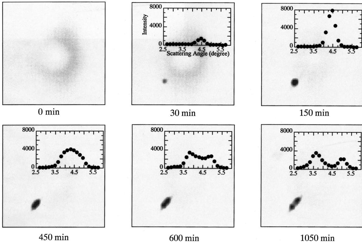
FIG. 3. Time resolved SANLD patterns for cubic phase at 46 °C transformed from lamellar phase in two dimensional expression. The insets show the intensity profiles along the radial principle axis.
