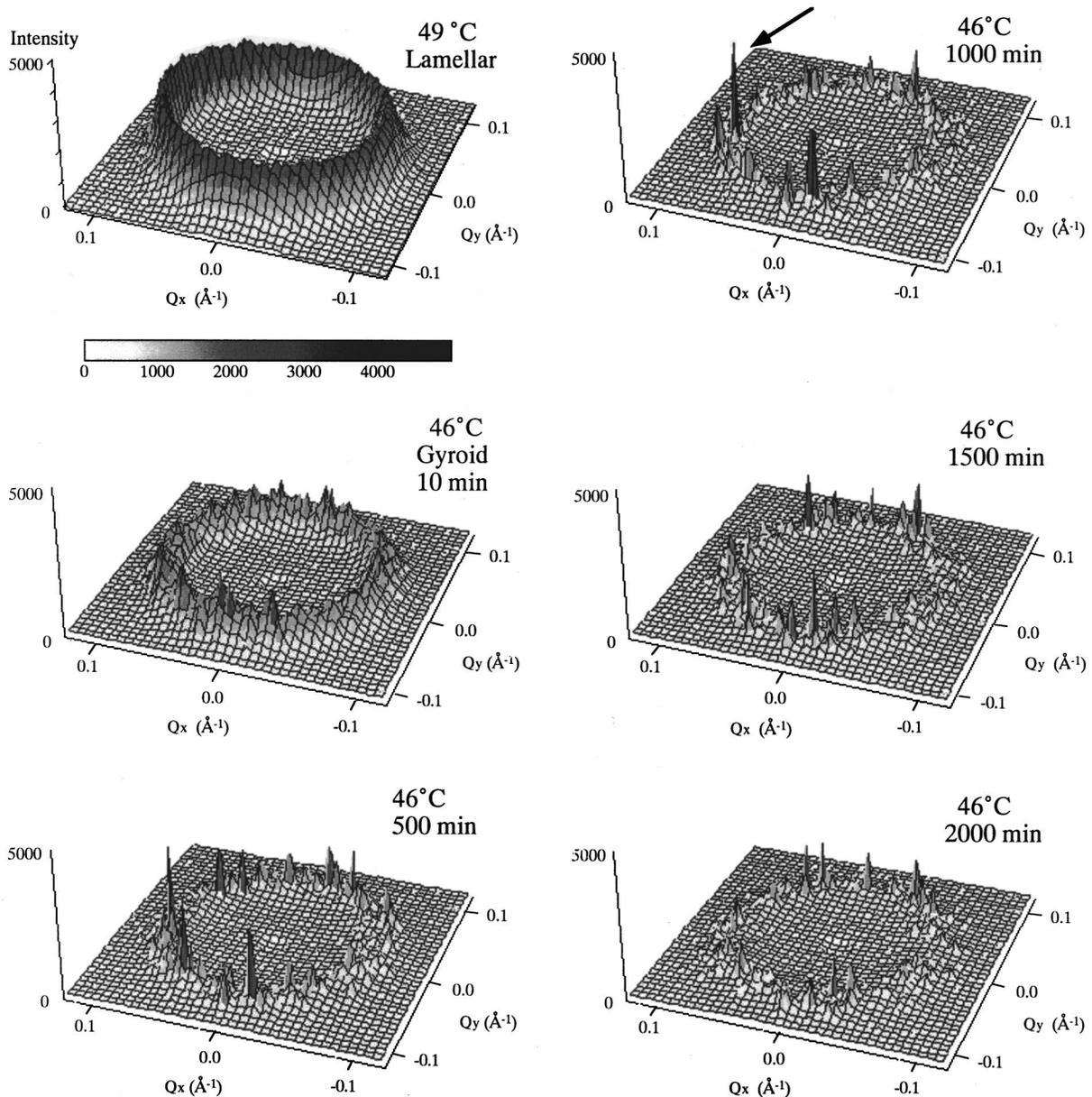
FIG. 1. Time resolved SANS patterns for cubic phase at 46 °C transformed from lamellar phase in two dimensional expression. The intensity and position of the peak marked by an arrow are plotted as a function of time in Figs. 2 and 5, respectively.
