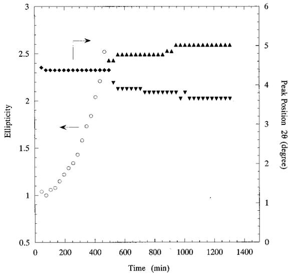
FIG. 4. Time dependence of the ellipticity and peak position of the Laue spots appearing in Fig. 3. Open circles denote the ellipticity and filled symbols (◆: before splitting and ▲, ▼: after splitting) denote the peak position.
