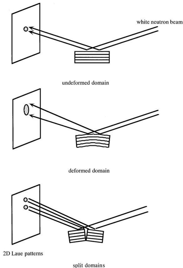
FIG. 6. Schematic representation of coarsening process of the gyroid domain with corresponding Laue patterns.
